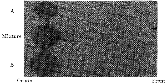
Plate 1. Mixed and parallel TLC bioautogram of subject urine (A) and N -demethyl-7-deoxy-7(S)-chlorolincomycin (B).
